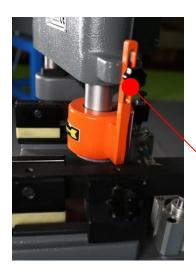
PROTECTION COVER LEVEL ADJUSTMENT SCREWS
