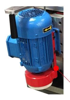
PROTECTION COVER LEVEL ADJUSTMENT SCREWS
